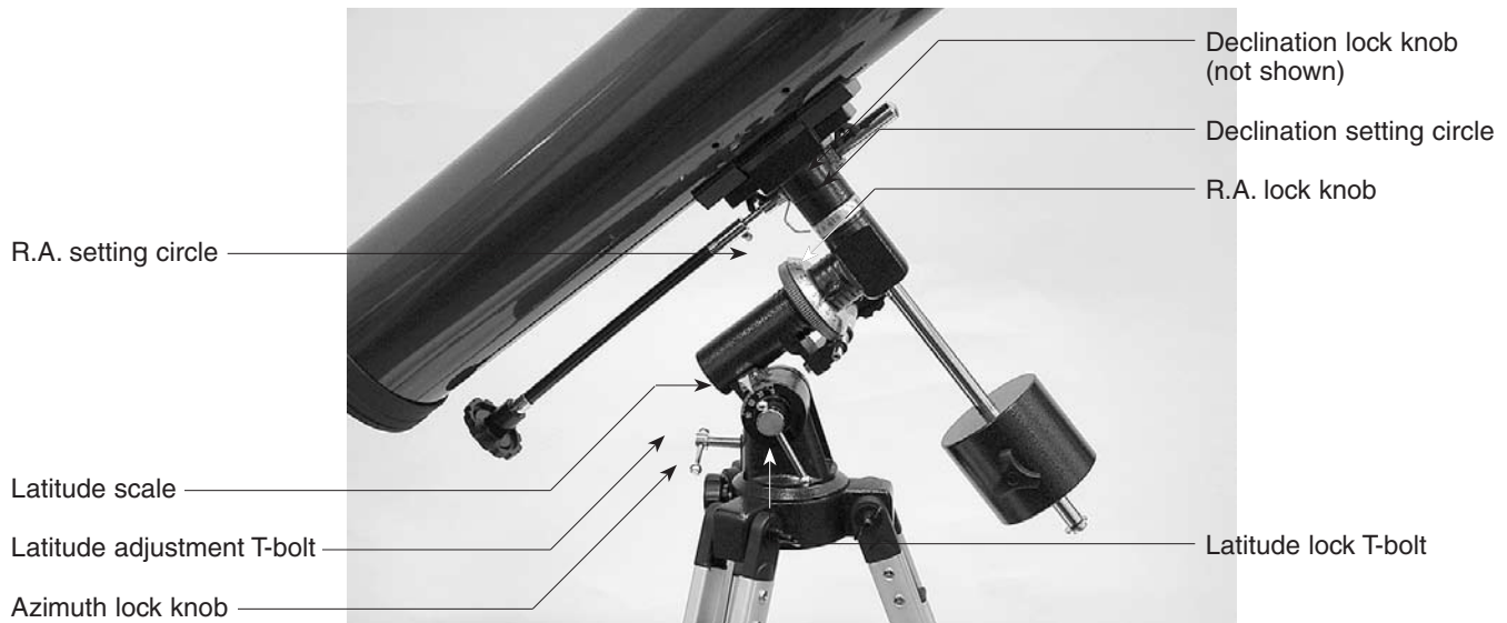
Figure 2. The equatorial mount of the SpaceProbe 3 EQ.
