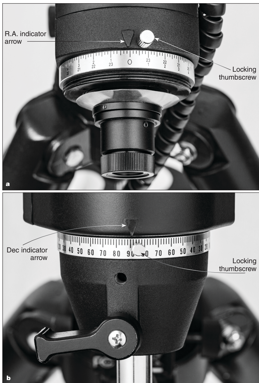
Figure 12. The RA and Dec setting circles ( a and b , respectively) can be used to locate objects manually by their coordinates, if desired.
