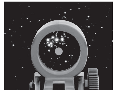
Figure 8: The Red-Dot finder superimposes a tiny red dot on the sky, showing right where the telescope is pointed.
