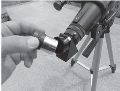
**Step 7:** Remove dust caps – on finder, the main telescope and eyepiece.
